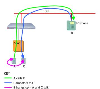
The Vega's default behaviour relies on detecting that two SIP call legs have the same call ID in order to initiate the QSIG side un-tromboning. Other headers can be checked and verified using the following parameters:
