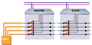
The status of the ISDN fallback relays can determine whether SIP registration takes place on a Vega E1T1 (models where ISDN fallback relays are fitted).
